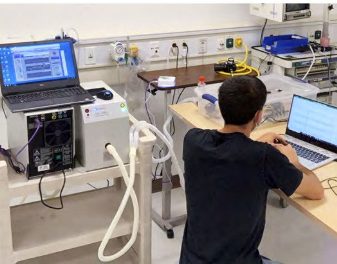
Using parts purchased from Home Depot, UCLA electrical and computer engineering graduate student and BioDesign Fellow Glen Meyerowitz built a prototype for a low-cost ventilator (top) that potentially could be employed in a hospital setting. He has gone on to refine his design (bottom left and right) and test it at the David Geffen School of Medicine at UCLA Simulation Center, using an artificial lung connected to the ventilator to determine the device's performance.
